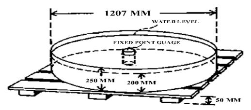
Figure 1. ClassA Evaporation Pan installed on a Wooden Platform
